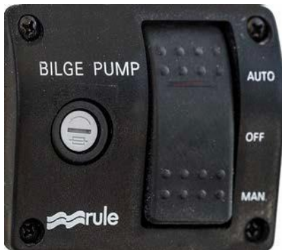
BILGE PUMP SWITCH
