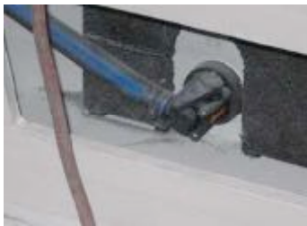
GENSET WATER SEPARATOR DISCHARGE THRU HULL Located outboard of engine compartment to starboard
