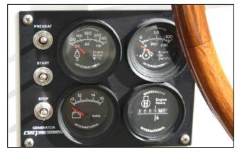
PREHEAT: Depress the PREHEAT switch first to activate control system
