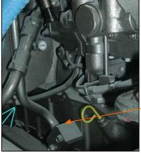
Engine Lube Oil Cooler (2 zincs) & 2<sup>nd</sup> Oil Dipstick (Starboard Forward)
