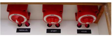
BATTERY SELECTOR SWITCHES A 4<sup>th</sup> Switch will be added if a Generator is Installed
