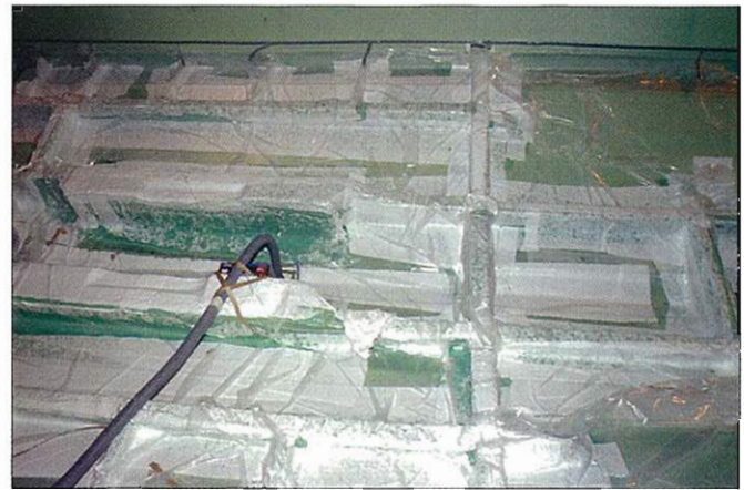
Left —Preassembled, precut lengths of three-ply stacked-and-sequenced process materials are located on a bench near the impregnator. Right —Moderate vacuum levels, combined with the controlled bleed of perforated release film, prevent absorption of excess resin into the bleeder. The soaked-through section in this image is over the thick engine-bed laminate region, and is normal.
