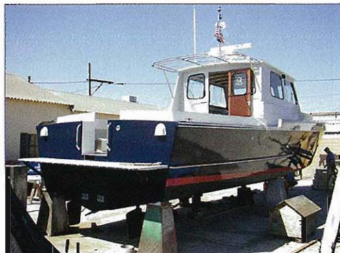
Top and above left —A recent Seaway build was this 40' (12.2m) cruising boat, using Stapp's proven construction methods. It's powered by twin 330-hp (246-kW) 5.9 BT Cummins diesels, and tops out at 28 knots. Above right —Bob Stapp founded Seaway Boats in Long Beach, California, nearly 50 years ago. Now, after delivering more than 160 durable glass-over-ply vessels, many to municipal agencies along the California coast, he'd like to sell the company and go fly-fishing.
