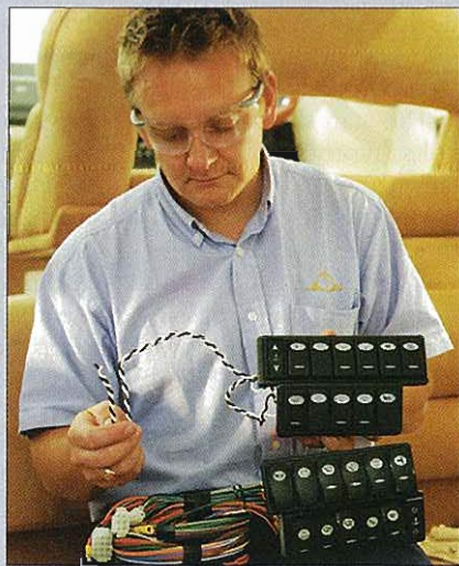
Julian Potter, manufacturing and engineering supervisor at Sealine, is outfitting selected models with an E-Plex power distribution system made by ED&D. Moving to networked marine systems constitutes a transformation, not just a changeover. At the helm alone, says Potter, one twisted-pair data/power cable (in his hand) has replaced two banks of seven switches and "an awful lot of wires."
