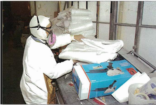
Left —Preassembled, precut lengths of three-ply stacked-and-sequenced process materials are located on a bench near the impregnator. Right —Moderate vacuum levels, combined with the controlled bleed of perforated release film, prevent absorption of excess resin into the bleeder. The soaked-through section in this image is over the thick engine-bed laminate region, and is normal.
