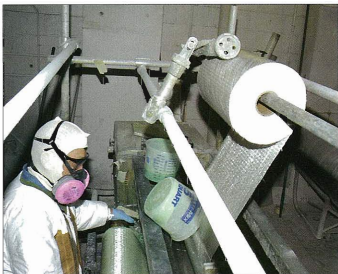
Above left —The machine operator, while manually rewinding wet-preg onto a cardboard core, looks up frequently at the footage counter on the unwind roll. Most rewind materials the author saw handed into the mold were precisely cut to length, with no end-trim required by the in-mold placement crew. Note that the wet-out material is being manually rewound onto the cardboard core, and that the roll of dry fiberglass above the nip is sitting off-center on the unwind arbor, with no side-stops or cone collars to align or center it. This setup works for low-to-moderate speeds—around 10–12 lineal feet (3m–3.7m) per minute. At faster speeds, not only will the rewind operator be unable to keep up, the unwound roll of dry fiberglass will start to wander from side to side. At that point, it's time to engage the air-operated rewinder, and fit the cone collars to align and center the unwound roll on its arbor.
