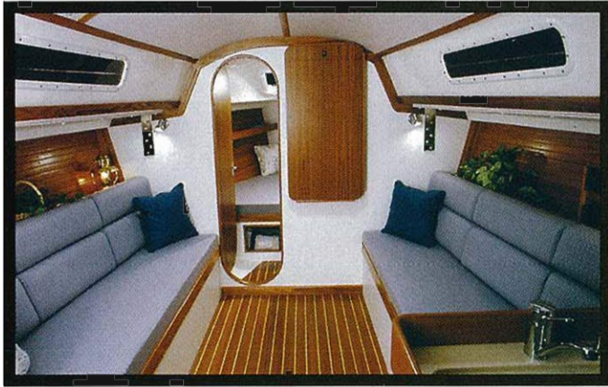
Left —The design of most J Boats begins with Rod Johnstone; the J/32, though, was designed entirely by his son Alan. Its varnished interior has 6'3" (1.9m) headroom. Right —The J/160 is one of several J Boat models intended more for cruising than racing. It features a three-cabin layout, a 7' (2.1m) retractable carbon fiber sprit for setting asymmetrical spinnakers, and can make upwind VMGs of 6.1 knots with a small jib.
